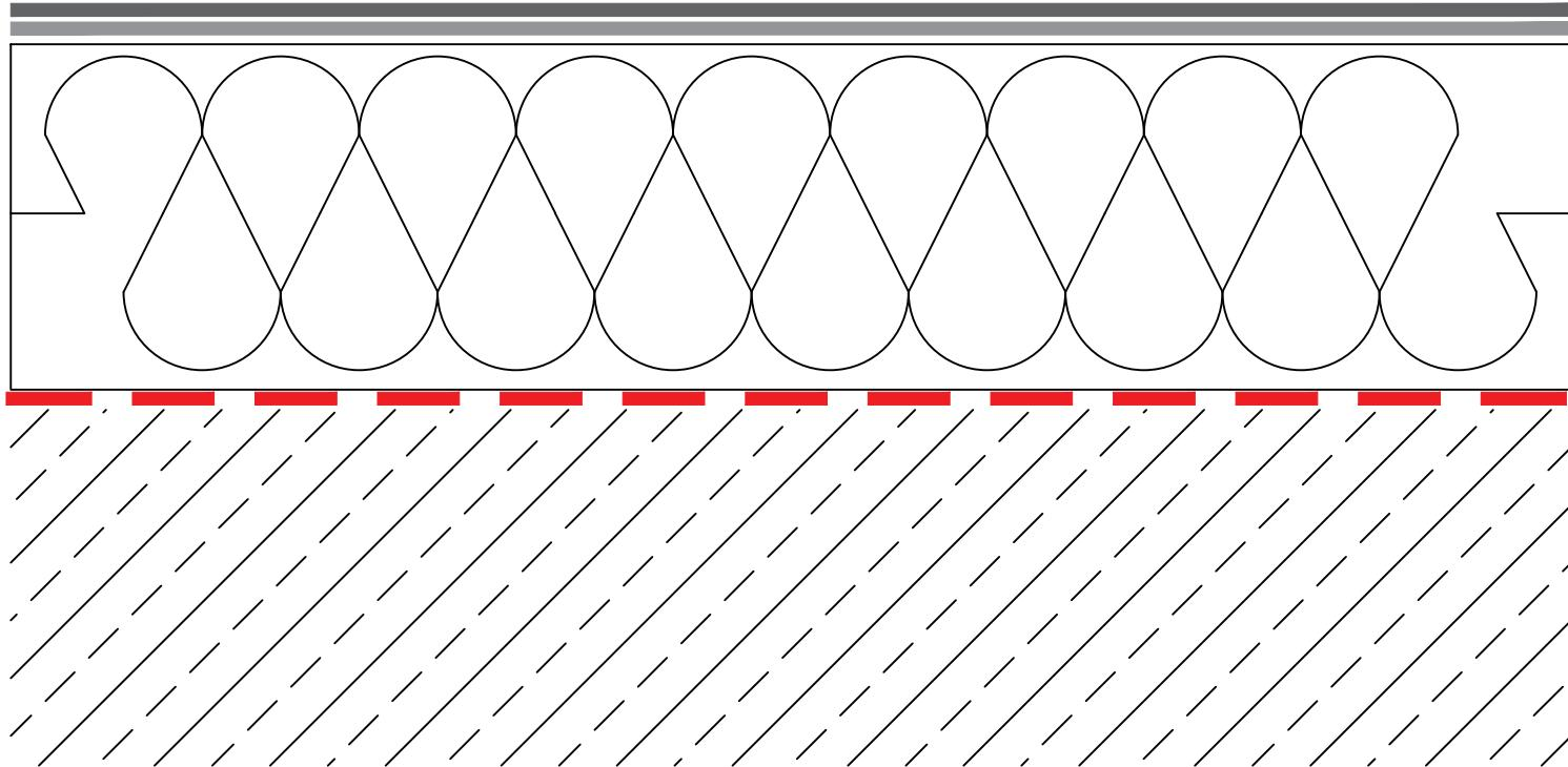
The Strata Pro M SA System has been independently tested against wind uplift forces. **The Strata Pro M SA System can be used on projects where the calculated wind loadings are 2.5kPa or lower.**
