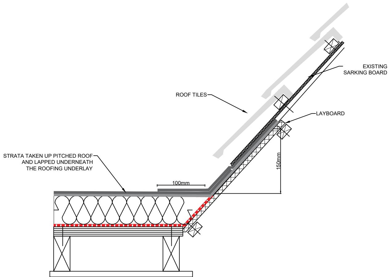
The Strata Pro M SA System has been independently tested against wind uplift forces. **The Strata Pro M SA System can be used on projects where the calculated wind loadings are 2.5kPa or lower.**
