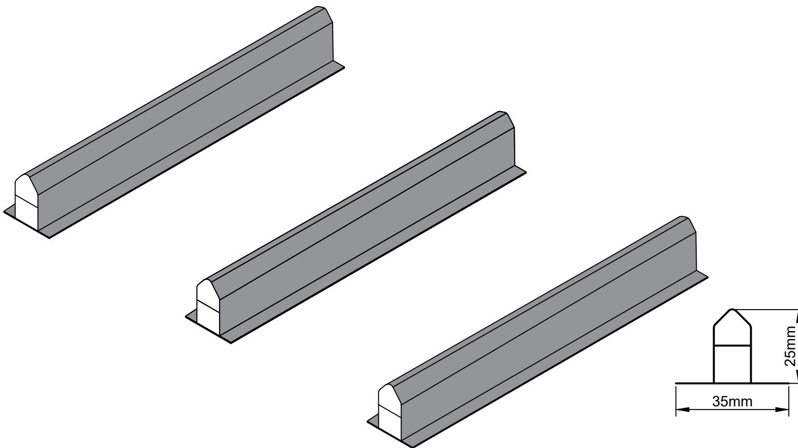
PVC Profile welded to Evalon membrane using liquid Evalon or Hot Air.
