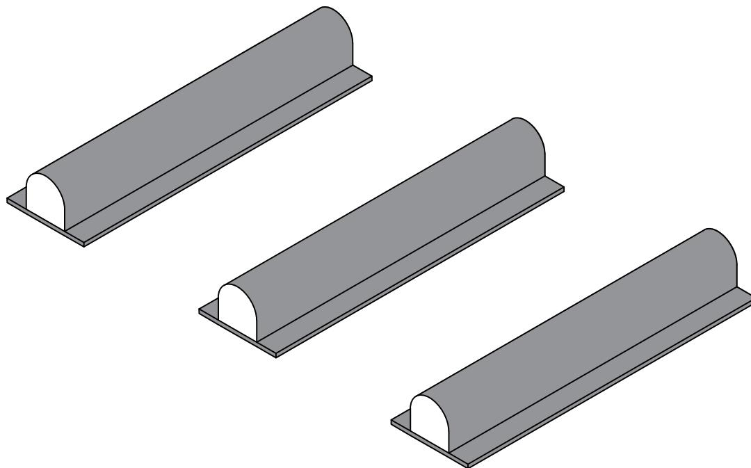
PVC Profile welded to Evalon membrane using liquid Evalon or Hot Air.
