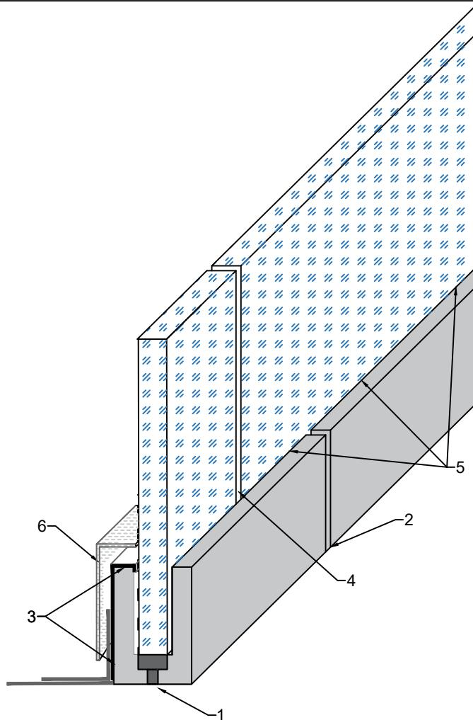
When installing a glass balustrade using an aluminium channel, there is always a chance of water ingress in vulnerable places, unless it is totally sealed.
