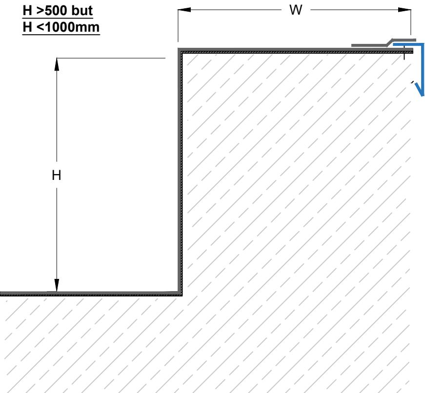
Where H is more than 500mm and less than 1000mm the membrane can be bonded using either:
