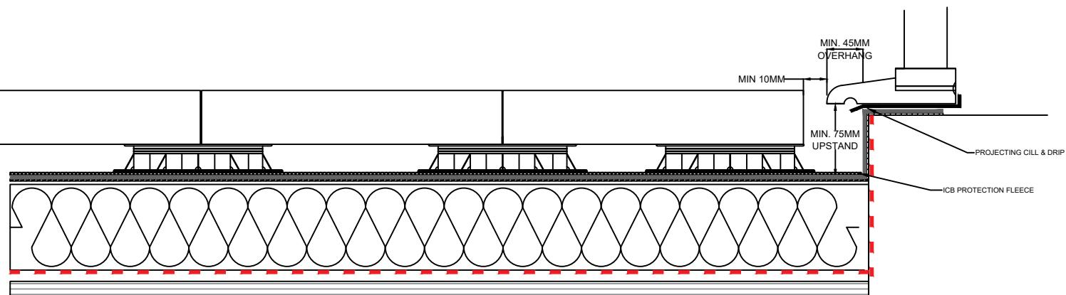
THE WATERPROOFING MEMBRANE MUST EXTEND 150MM HIGH IN THE DOOR REVEAL / ROOF OR WALL ABUTMENT.
