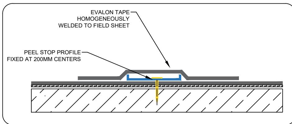
Note: Peel stop profiles must be used in situations where the calculated wind pressure will be above 2.4 KM/m<sup>2</sup>. Additionally peel stops must be used in vertical upstands over 800mm + and repeated every 300mm.
